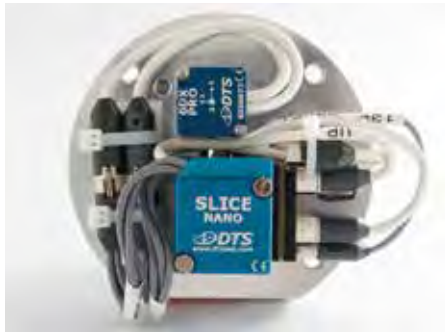
RIGHT: DTS offers mounting brackets with proper CG to embed both the sensors and even Slice Nano miniature recorders in dummy heads, free motion headforms and pedestrian headforms
