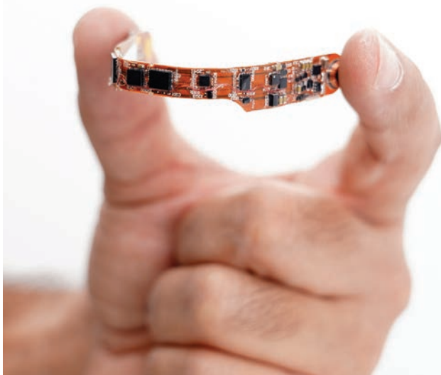
The DTS DDR is a miniature 6DOF dosimeter featuring triaxial linear and angular accelerometers
