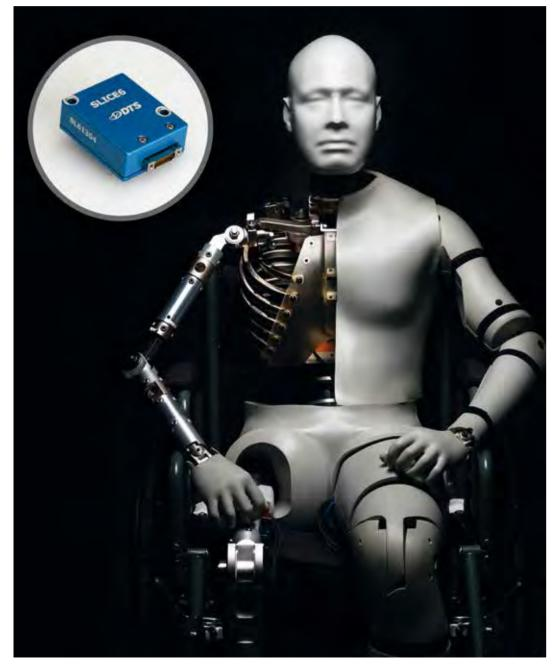
Frontal, side and rear impacts are assessed as standard in automotive crash testing, but vertical loads are also a factor, particularly when it comes to testing military or armored vehicles for diplomatic and high-asset personnel. Data shows that secondary blast injuries are more common than primary ones. As long as the hull has not been breached, many critical injuries are caused by that secondary impact when the vehicle lands or by debris that is displaced by the blast wind of the explosion.
