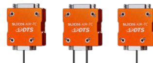
SLICE6 AIR-TC data acquisition unit with three TC Interface blocks, shown as a 24-channel system
